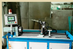
Gas burner pipe CNC drilling machine (5set)
